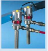
This assembly allows a small quantity of each component to be dispensed in an amount corresponding to the mixing ratio. These materials may then be mixed manually for touch-ups, which is very advantageous. No additional cleaning is necessary, as each component is dispensed separately.
