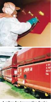
A railcar for transporting food is being coated with a solvent-free, thick polyurethane coating using a WIWA DUOMIX 333 (solids: 92,5%, potlife: 5 minutes, spraying temperature: 60°C).
