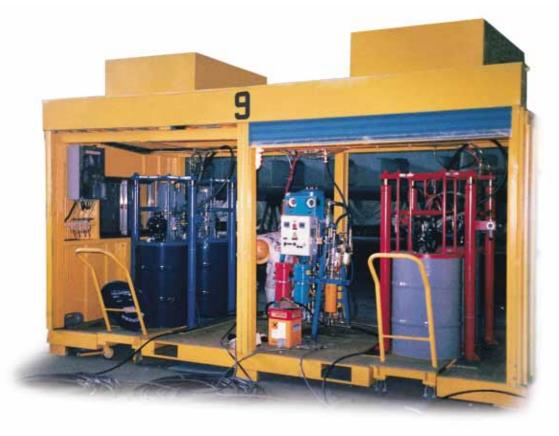
A complete WIWA DUOMIX Dual Component Unit, including an automatic drum refill system for both the base and hardener components, is integrated in a container, providing security, mobility and a miximum utilization of space. This enables the operator to quickly change locations within the wharf or on a shipdeck. Futhermore, the system is protected against climatic influences, as well as unauthorized access.
