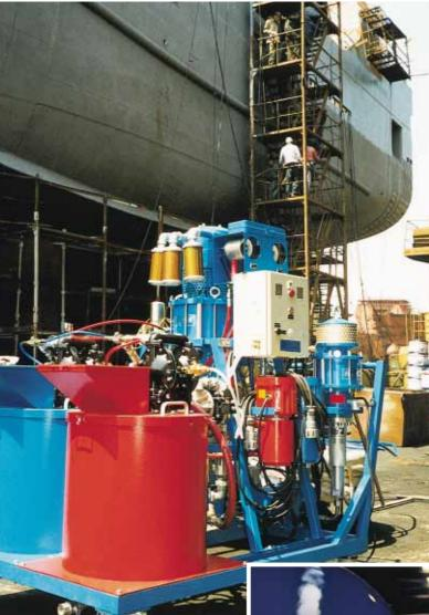
Here, **an icebreaker** is being sprayed with a special coating material (potlife: 5 minutes, spraying temperature: 55°C) using a WIWA DUOMIX 333 with heated hoses.
