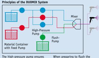
that the exact dosage of each coating material component (base and hardener) is dispensed into the mixing block and then led to the spraying gun.
