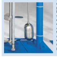
In order to achieve interruption-free operation of the WIWA DUOMIX Dual Component Spraying System, either a pneumatic or electric drum level indicator should be installed to monitor the amount of material remaining in each drum. When using the WIWA automatic drum refilling system, the feed drum is refilled automatically from a second drum once the level indicator registers that the minimum point has been reached.
